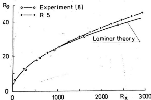
**Figure 2:** Stream wise growth of momentum thickness  $\theta(x), R_\theta, R_x$ ; laminar Reynolds range
