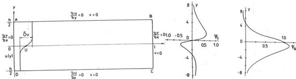
**Figure 1:** Left: Simulation domain geometry and steady boundary conditions Right: Eigen-functions of most unstable disturbance from Michalke
