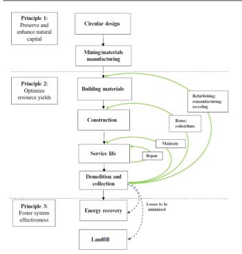
**Figure 1:** Basic concepts for handling the CE adoption in the operational cycle of construction value chain[3]
