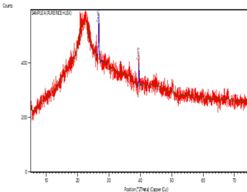
Figure 5: XRD result of Sample A
