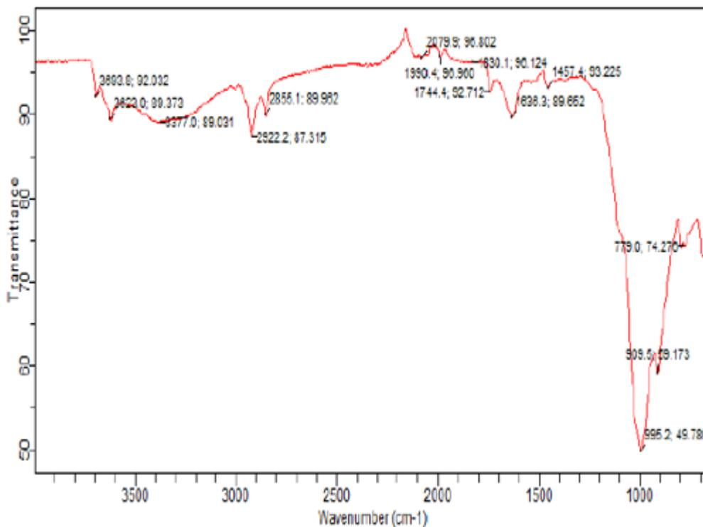
Figure 4: FTIR analysis of Rice husk + Bentonite clay (2:1), Sample D
