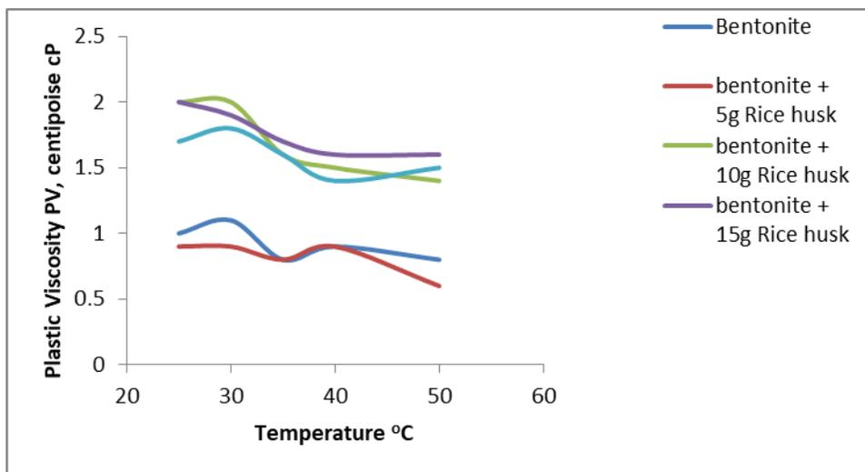
**Figure 9:** Plastic viscosity of samples against Temperature for Samples 1 to 5
