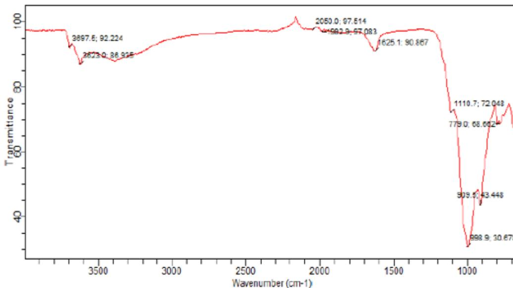
Figure 2: FTIR analysis of pure Bentonite clay, Sample B
