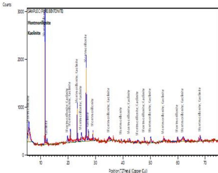
Figure 6: XRD result of Sample B
