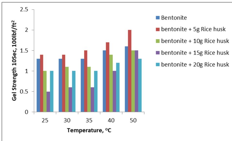
**Figure 11:** Gel strengths (10 secs) for the five samples at various temperatures
