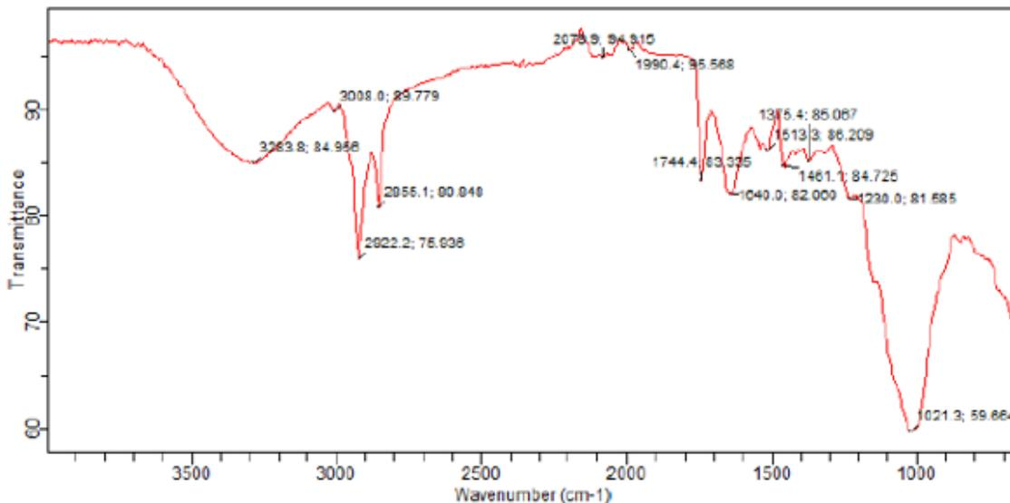
Figure 1: FTIR analysis of pure Rice husk, Sample A
