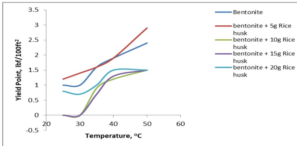
**Figure 10:** Yield point against temperature for Samples 1 to 5
