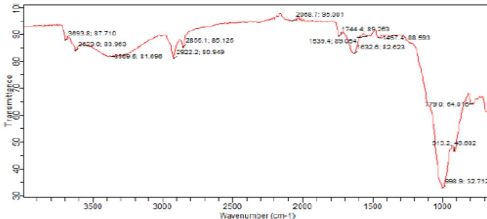
Figure 3: FTIR analysis of Rice husk + Bentonite clay (1:1), Sample C
