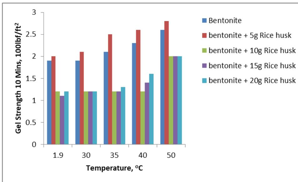
**Figure 12:** Gel strengths (10 minutes) for the five samples at various temperatures
