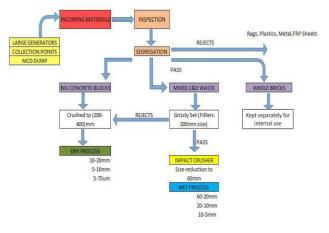
Figure 9: Recycling process
