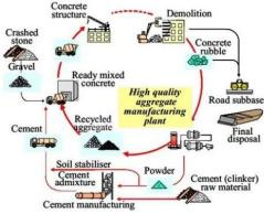
Figure 8: Concrete recycling process
