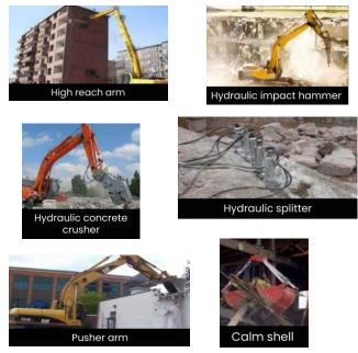
Figure 7: Types of demolition equipment
