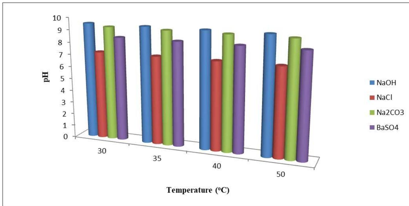
Figure 16: Variation of pH with temperature for Sample B with 3.5g each of (NaOH, NaCl, Na<sub>2</sub>CO<sub>3</sub>) and 17.5g of BaSO<sub>4</sub>
