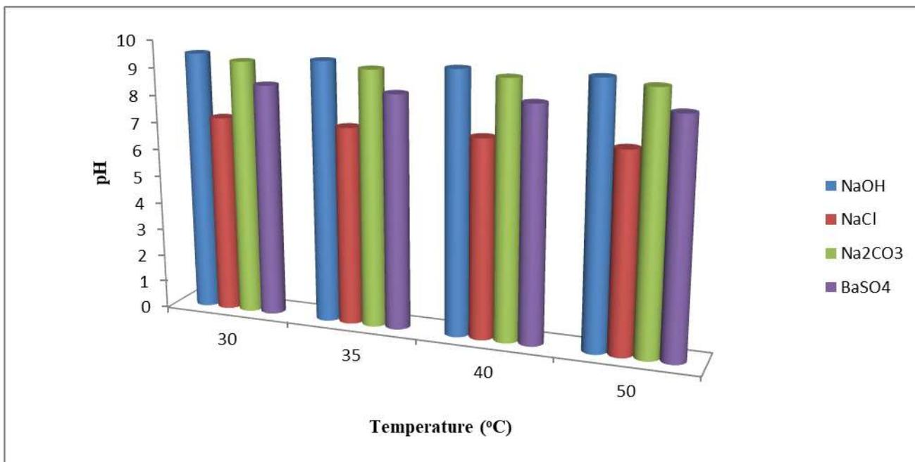
Figure 17: Variation of pH with temperature for Sample B with 7g each of (NaOH, NaCl, Na<sub>2</sub>CO<sub>3</sub>) and 35g of BaSO<sub>4</sub>
