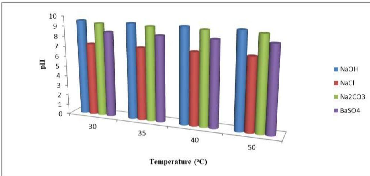
Figure 18: Variation of pH with temperature for Sample B with 10.5g each of (NaOH, NaCl, Na<sub>2</sub>CO<sub>3</sub>) and 52.5g of BaSO<sub>4</sub>
