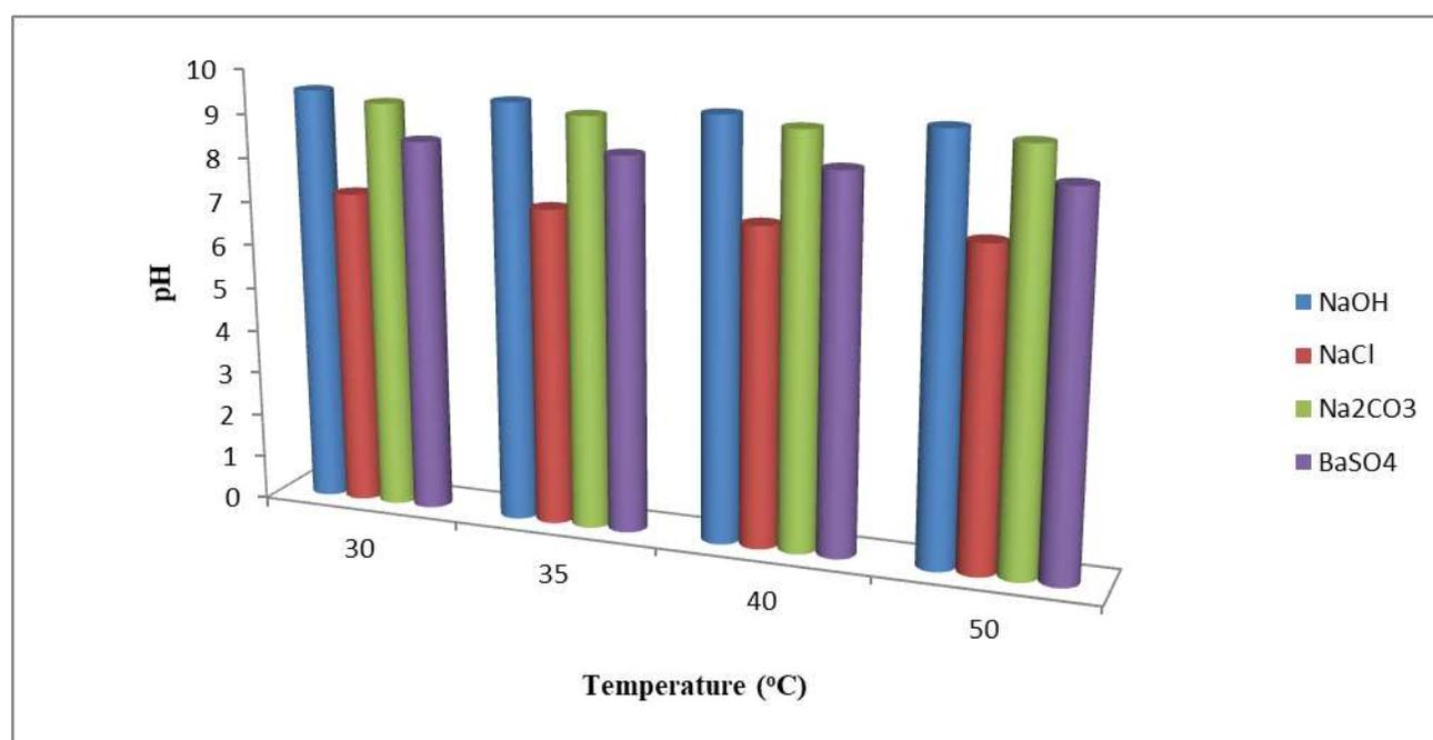
**Figure 20:** Variation of pH with temperature for Sample C with 7g each of (NaOH, NaCl, Na<sub>2</sub>CO<sub>3</sub>) and 35g of BaSO<sub>4</sub>
