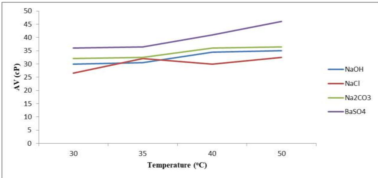
**Figure.12:** Variation of Apparent viscosity with temperature for Sample D with 10.5g each of (NaOH, NaCl, Na<sub>2</sub>CO<sub>3</sub>) and 52.5g of BaSO<sub>4</sub>
