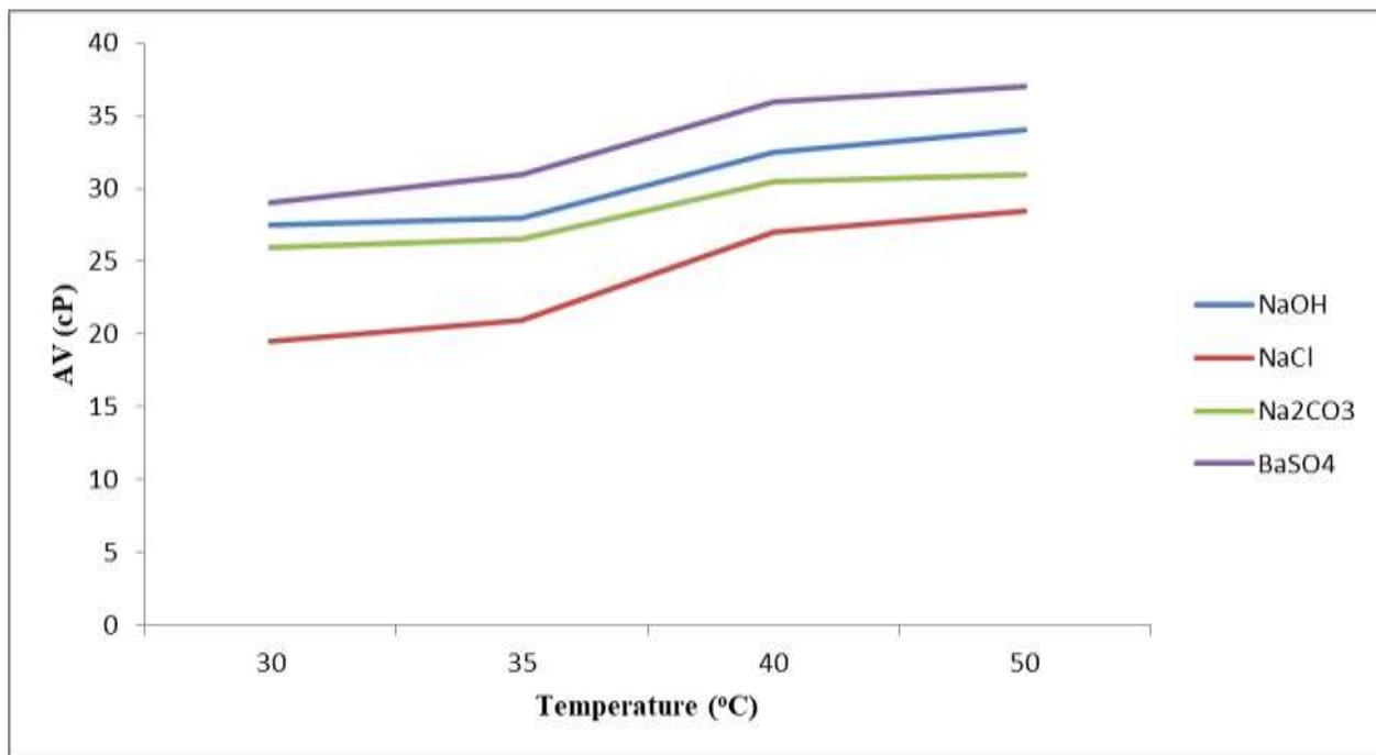
**Figure 9:** Variation of Apparent viscosity with temperature for Sample C with 10.5g each of (NaOH, NaCl, Na<sub>2</sub>CO<sub>3</sub>) and 52.5g of BaSO<sub>4</sub>
