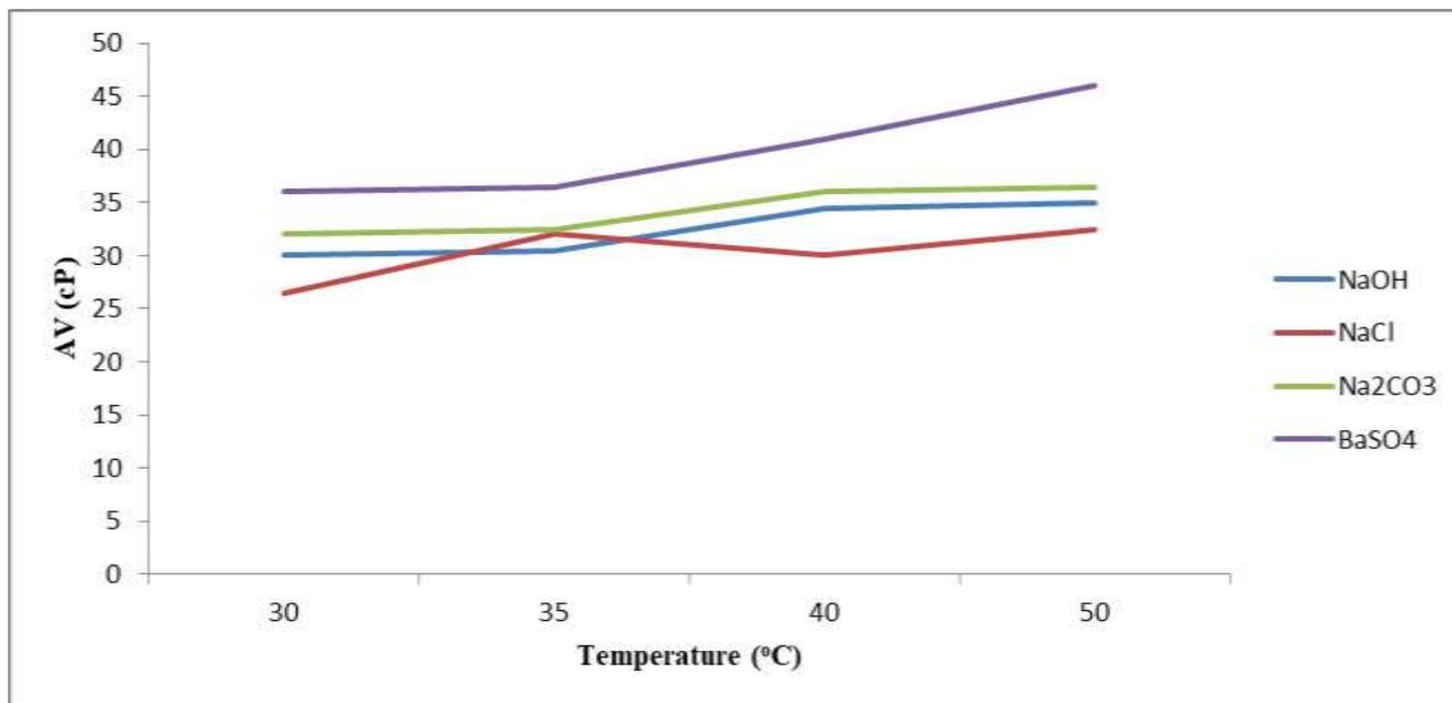
**Figure 11:** Variation of Apparent viscosity with temperature for Sample D with 10.5g each of (NaOH, NaCl, Na<sub>2</sub>CO<sub>3</sub>) and 52.5g of BaSO<sub>4</sub>
