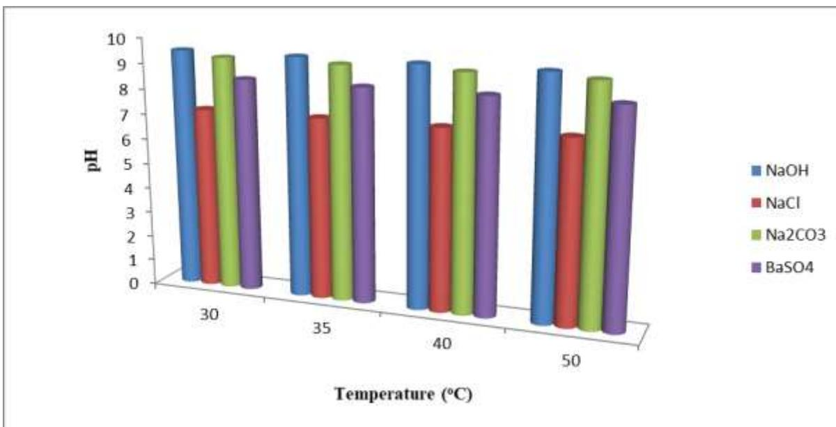
**Figure 14:** Variation of pH with temperature for Sample A with 7g each of (NaOH, NaCl, Na<sub>2</sub>CO<sub>3</sub>) and 35g of BaSO<sub>4</sub>
