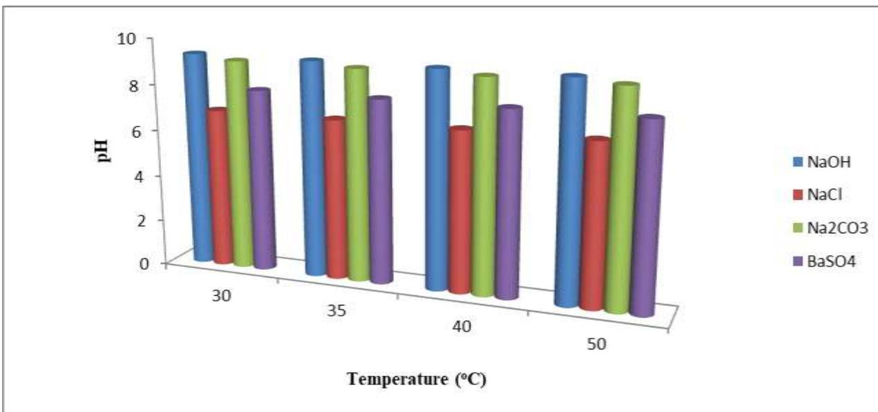
Figure 24: Variation of pH with temperature for Sample D with 10.5g each of (NaOH, NaCl, Na<sub>2</sub>CO<sub>3</sub>) and 52.5g of BaSO
