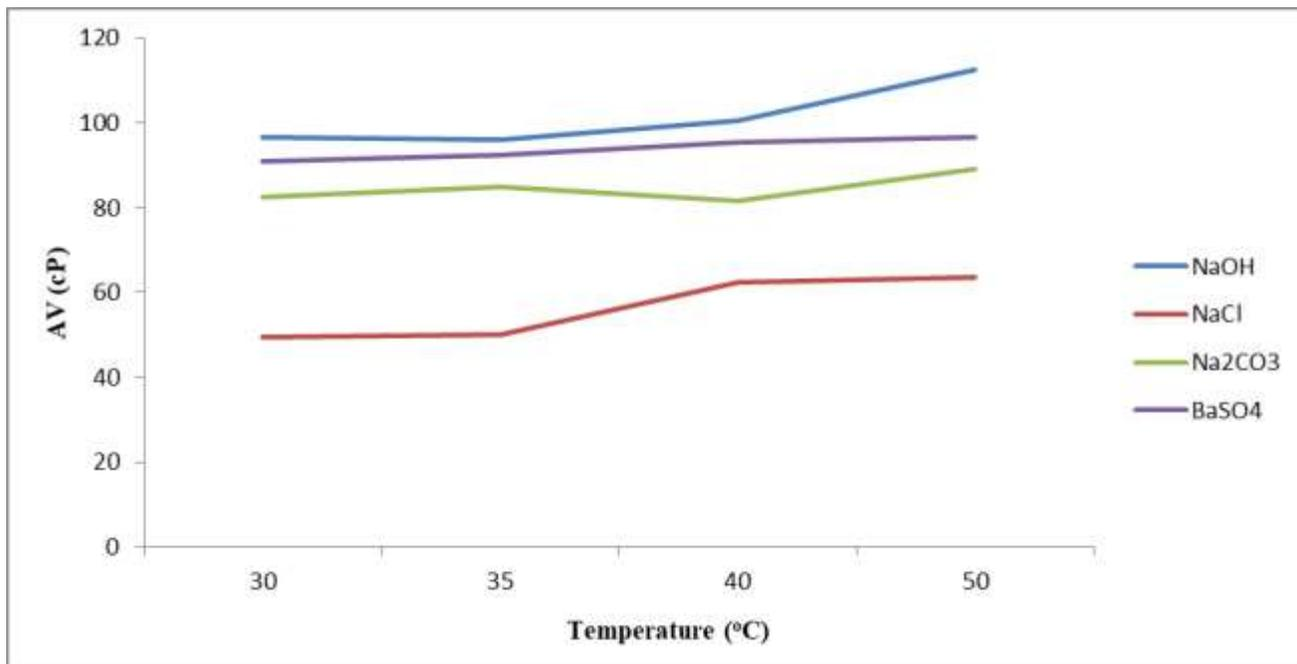
**Figure 3:** Variation of Apparent viscosity with temperature for Sample A with 10.5g each of (NaOH, NaCl, Na<sub>2</sub>CO<sub>3</sub>) and 52.5g of BaSO<sub>4</sub>
