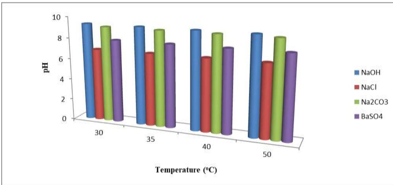
Figure 22: Variation of pH with temperature for Sample D with 3.5g each of (NaOH, NaCl, Na<sub>2</sub>CO<sub>3</sub>) and 17.5g of BaSO<sub>4</sub>
