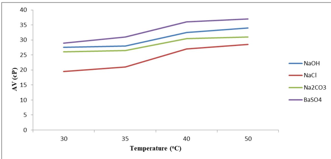
**Figure 8:** Variation of Apparent viscosity with temperature for Sample C with 7g each of (NaOH, NaCl, Na<sub>2</sub>CO<sub>3</sub>) and 35g of BaSO<sub>4</sub>
