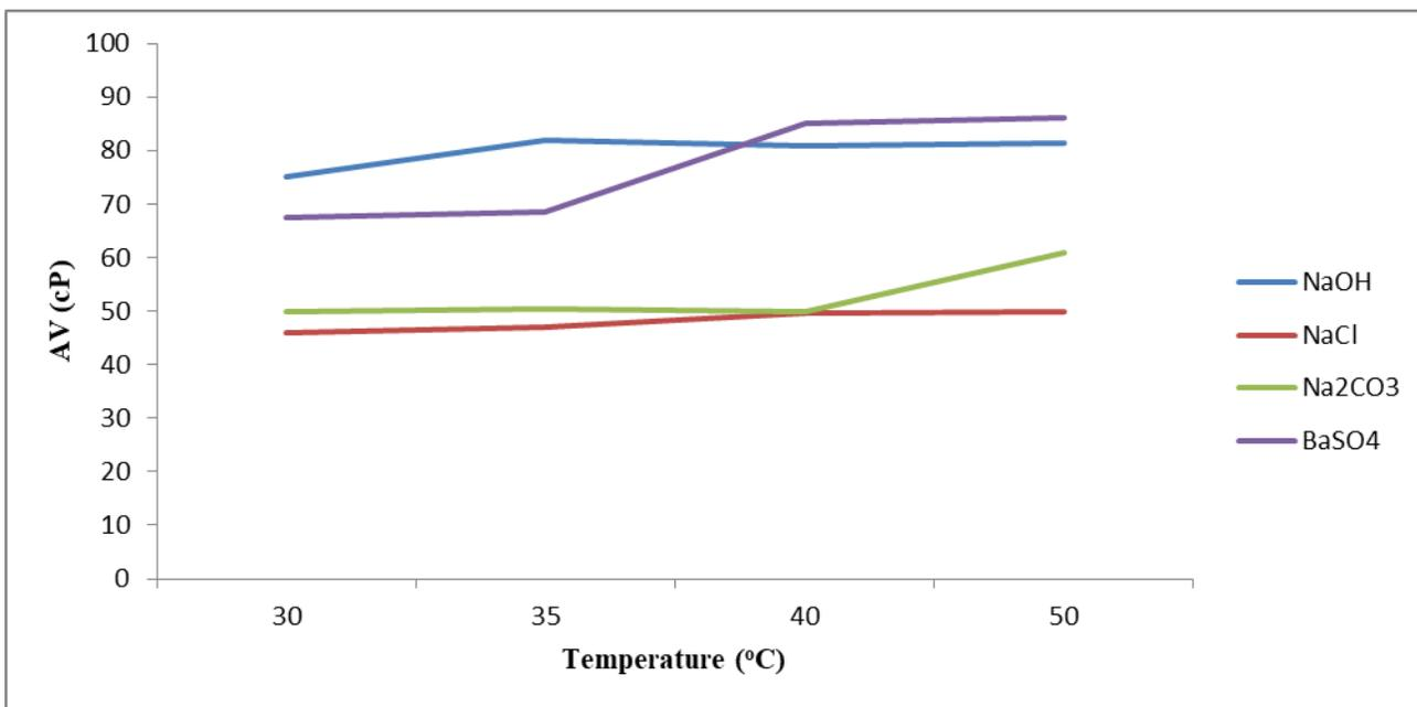
**Figure 6:** Variation of Apparent viscosity with temperature for Sample B with 10.5g each of (NaOH, NaCl, Na<sub>2</sub>CO<sub>3</sub>) and 52.5g of BaSO<sub>4</sub> 0
