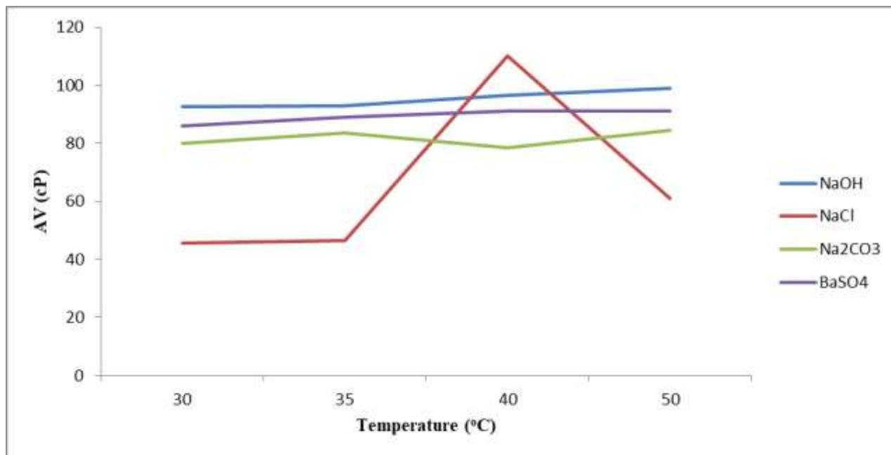
**Figure 2:** Variation of Apparent viscosity with temperature for Sample A with 7g each of (NaOH, NaCl, Na<sub>2</sub>CO<sub>3</sub>) and 35g of BaSO<sub>4</sub>
