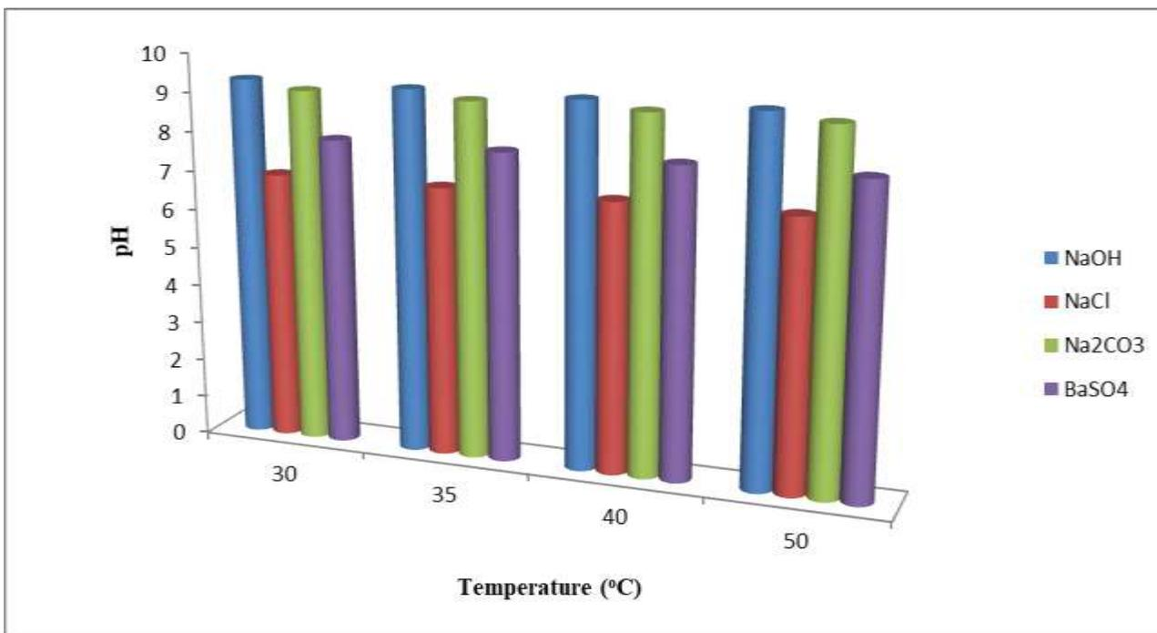
Figure 23: Variation of pH with temperature for Sample D with 7g each of (NaOH, NaCl, Na<sub>2</sub>CO<sub>3</sub>) and 35g of BaSO<sub>4</sub>
