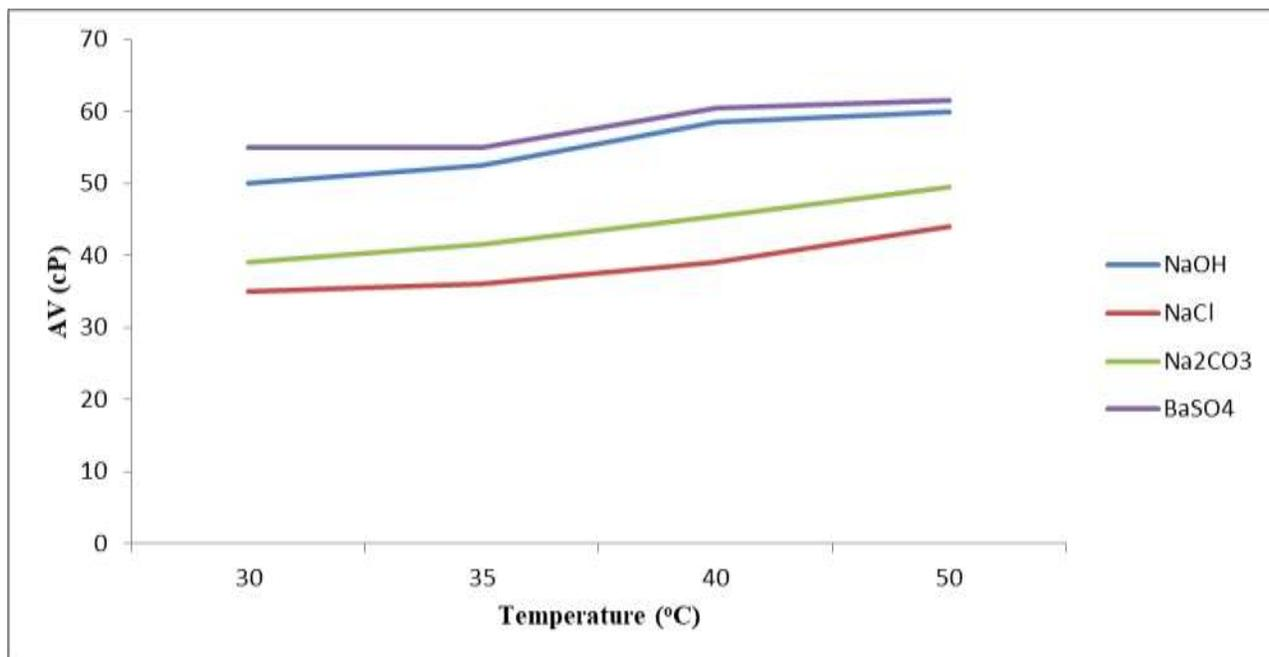
**Figure 4:** Variation of Apparent viscosity with temperature for Sample B with 3.5g each of (NaOH, NaCl, Na<sub>2</sub>CO<sub>3</sub>) and 17.5g of BaSO<sub>4</sub>
