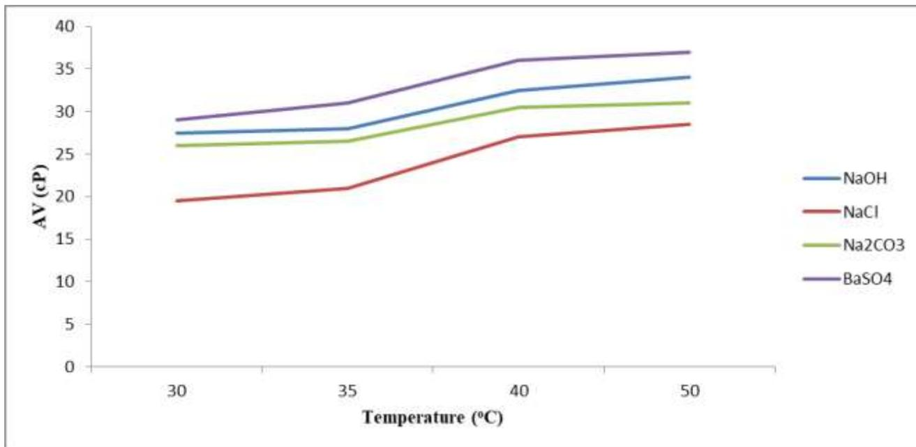
**Figure 7:** Variation of Apparent viscosity with temperature for Sample C with 3.5g each of (NaOH, NaCl, Na<sub>2</sub>CO<sub>3</sub>) and 17.5g of BaSO<sub>4</sub>
