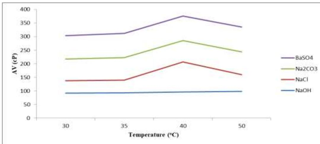
**Figure 1:** Variation of Apparent viscosity with temperature for Sample A with 3.5g each of (NaOH, NaCl, Na<sub>2</sub>CO<sub>3</sub>) and 17.5g of BaSO<sub>4</sub>
