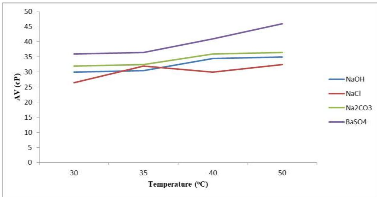
**Figure 10:** Variation of Apparent viscosity with temperature for Sample D with 3.5g each of (NaOH, NaCl, Na<sub>2</sub>CO<sub>3</sub>) and 17.5g of BaSO<sub>4</sub>
