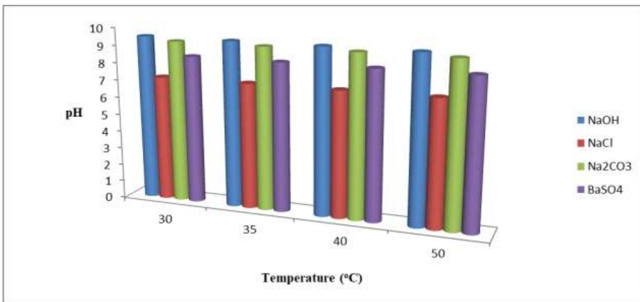
**Figure 13:** Variation of pH with temperature for Sample A with 3.5g each of (NaOH, NaCl, Na<sub>2</sub>CO<sub>3</sub>) and 17.5g of BaSO<sub>4</sub>
