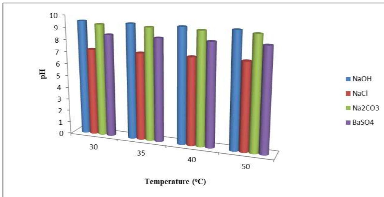
Figure 21: Variation of pH with temperature for Sample C with 10.5 each of (NaOH, NaCl, Na<sub>2</sub>CO<sub>3</sub>) and 52.5g of BaSO<sub>4</sub>
