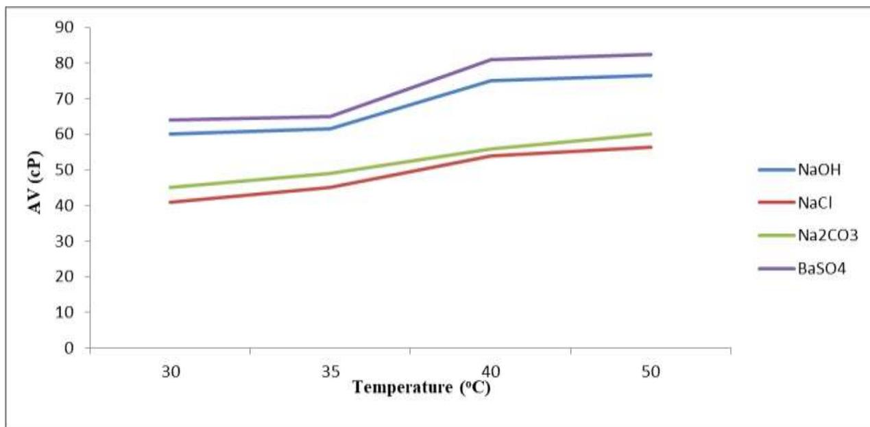
**Figure 5:** Variation of Apparent viscosity with temperature for Sample B with 7g each of (NaOH, NaCl, Na<sub>2</sub>CO<sub>3</sub>) and 35g of BaSO<sub>4</sub>
