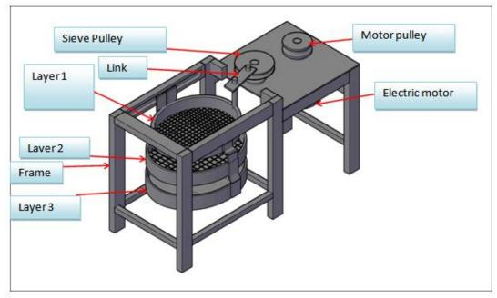
Figure 1: Isometric view of the fabricated machine
