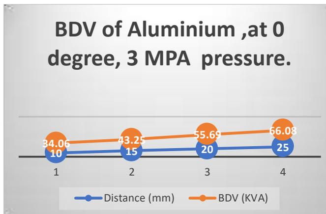
**Figure 10:** Variation of N<sub>2</sub> gas breakdown voltage of Aluminium metal for the Plane-Plane electrode combination (0°)
