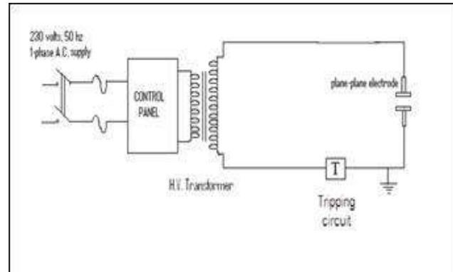
**Figure 3:** Circuit Diagram for HVAC System
