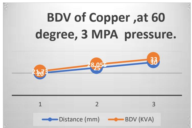
**Figure 9:** Variation of N<sub>2</sub> gas breakdown voltage of Copper metal for the Plane-Plane electrode combination (60°)
