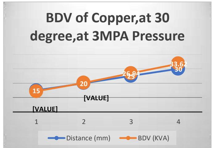
**Figure 8:** Variation of N<sub>2</sub> gas breakdown voltage of Copper metal for the Plane-Plane electrode combination (30°)
