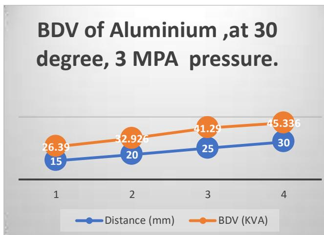
**Figure 11:** Variation of N<sub>2</sub> gas breakdown voltage of Aluminium metal for the Plane-Plane electrode combination (30°)
