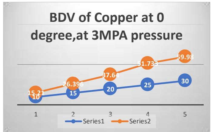
**Figure 7:** Variation of N<sub>2</sub> gas breakdown voltage of Copper metal for the Plane-Plane electrode combination (0°)
