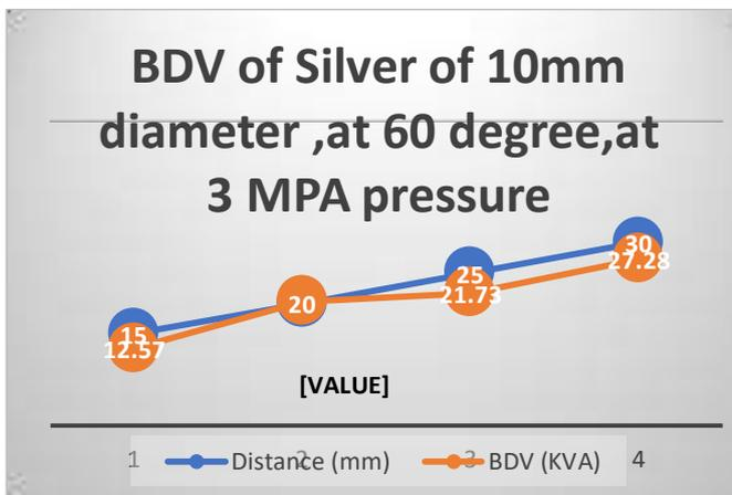
**Figure 6:** Variation of N<sub>2</sub> gas breakdown voltage of Silver metal for the Plane-Plane electrode combination (60°)
