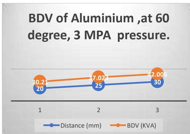
**Figure 12:** Variation of N<sub>2</sub> gas breakdown voltage of Aluminium metal for the Plane-Plane electrode combination (60°)
