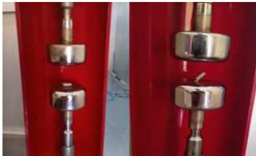
**Figure 1:** Plane-Plane electrode arrangements with metal placed in angles 0°, 30°, 60°
