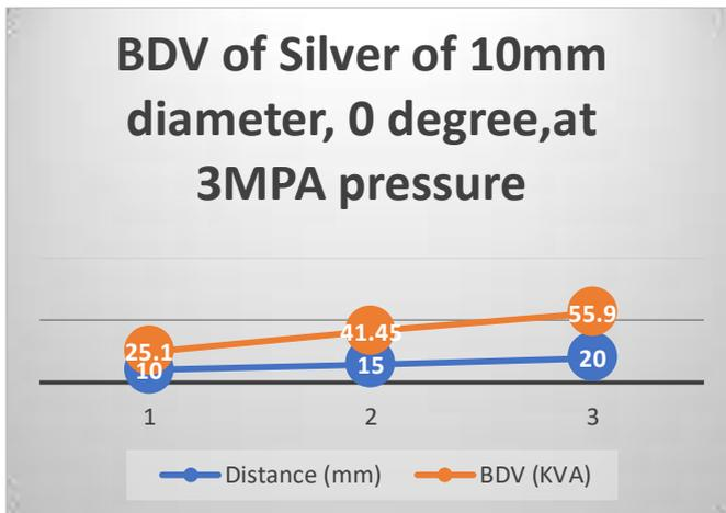
**Figure 4:** Variation of N<sub>2</sub> gas breakdown voltage of Silver metal for the Plane-Plane electrode combination (0°)
