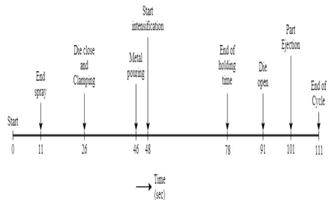
Figure 2: Die casting heat cycle process cycle represented on a timeline in seconds (Industrial case-CGL)
