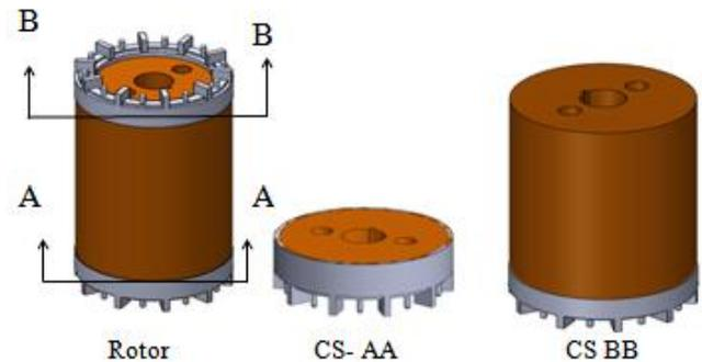
Figure 1: Die casting rotor component and cs at AA and BB for numerical analysis
