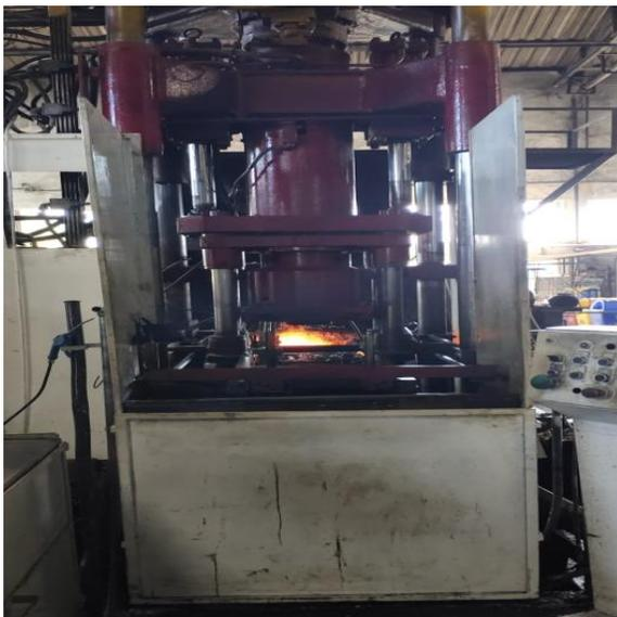
**Figure 3:** Experimentation setup: vertical die casting machine of the capacity of 100 Tons (Industrial case-CGL)
