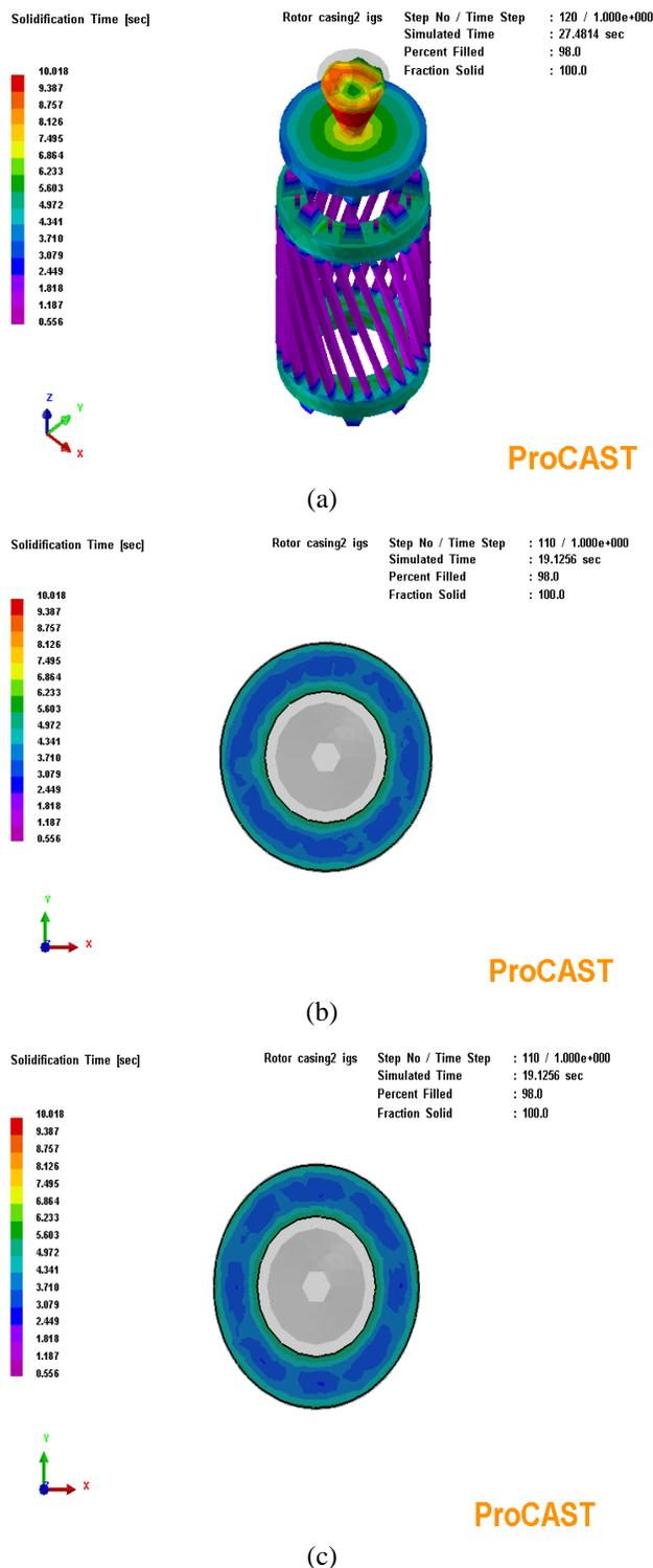
Figure 15: (a, b, and c) Simulation output for solidification time at rotor component, Cross-Section AA and BB.
