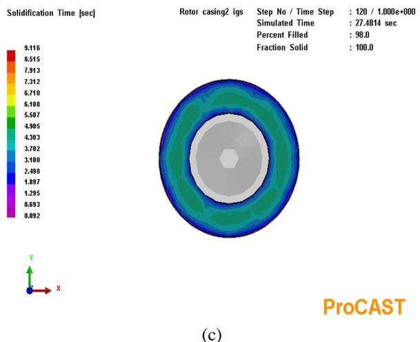
**Figure 13:** (a, b, and c) Simulation output for solidification time at rotor component, Cross-Section AA and BB.
