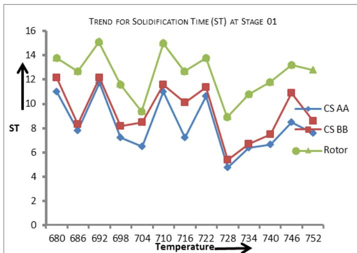
**Figure 8:** Graphical representation of temperature analysis of the rotor and at cross-sections AA and BB
