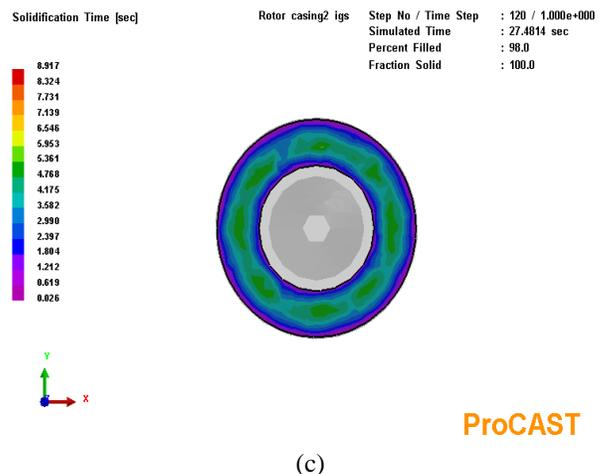
Figure 11: (a, b, and c). Simulation output for solidification time at rotor component, Cross-Section AA, and BB.
