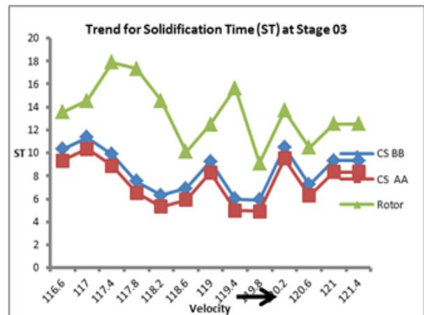
**Figure 12:** Graphical representation of plunger velocity analysis at various sections
