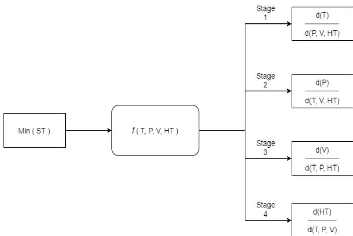
Figure 5: Block diagram showing four stages of numerical simulation for the optimisation of solidification time
