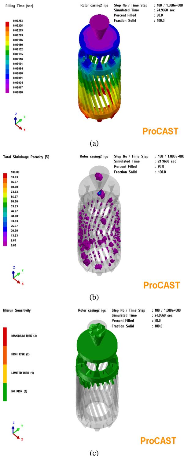
**Figure 16:** (a, b, c,) ProCAST simulated results for filling time, total shrinkage porosity and misrun sensitivity
