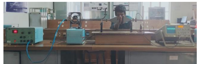
Figure9: Experimental setup for return loss measurement with obstacle
