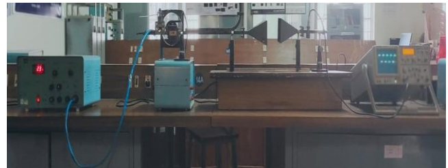
Figure 8: Experimental setup for return loss measurement without obstacle
