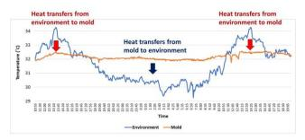
Figure 5: Fluctuation of the direction of heat transfer between mold and environment
