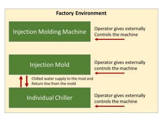
Figure 6: Stansalone arrangement of the Injection Mold Machine setup
