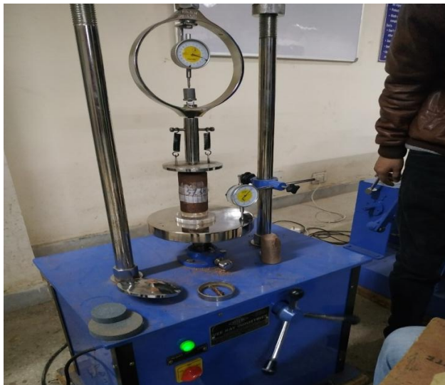
Unconfined Strength Testing Machine
