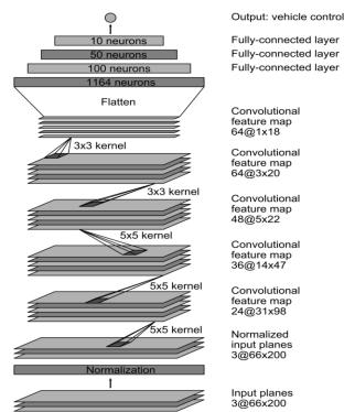
Figure 3: NVIDIA Convolutional Neural Network [13]
