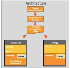
Figure 5: TensorFlow Lite architecture [19]
