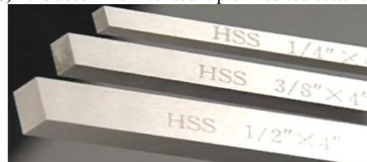
Fig. - 2: HSS Cutting Tool
