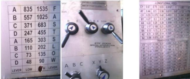
Fig. -3: (a) Selected Cutting Speed (rpm) (b) Selected Feed Rate (mm/min)
