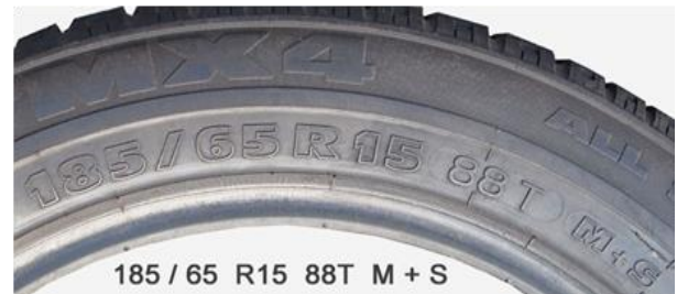
Figure 1: Tyre Image Showing Tyre Markings
