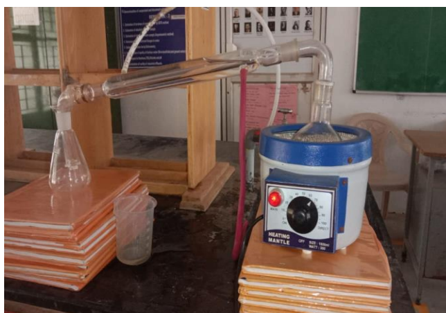
Figure 3: Simple distillation process for extraction of oil
