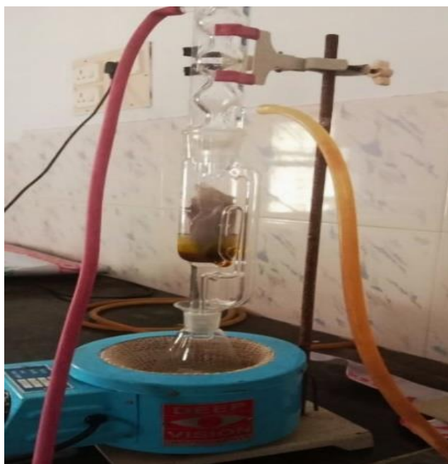
Figure 2: Experimental setup for extraction of the solution from the raw material
