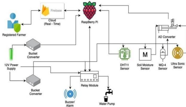
Figure 5: Smart Irrigation System
