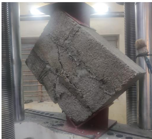
Figure 1: Crack pattern of diagonal compressive strength
