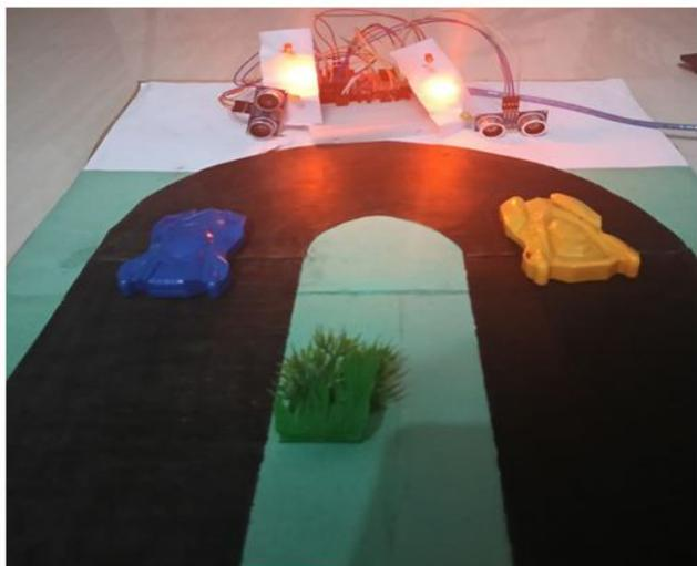
**Figure 5:** When two cars are reached to very near-by distance red color LED lights are blinked to alert the danger.
