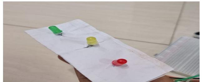
In our project, we utilized three LEDs: red, green, and yellow. As depicted in the illustration, the longer leg of the LED serves as the positive terminal (anode), while the shorter leg functions as the negative terminal (cathode). These three LEDs are employed to signal the location and distance of an oncoming vehicle. Two sets of LEDs need to be linked to the ground using jumper wires.
