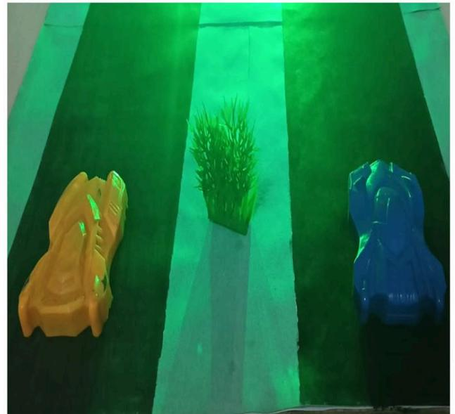
**Figure 2:** If there is only one car on the road, a green LED light on the same side will blink, while a yellow LED light on the opposite side will blink to alert oncoming vehicles.
